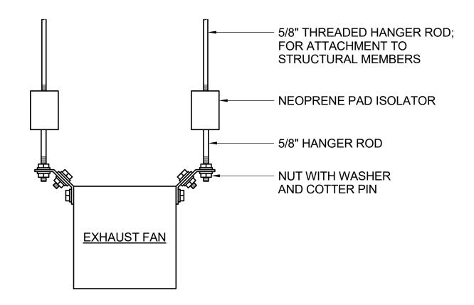
INLINE EXHAUST FAN MOUNTING DETAIL
